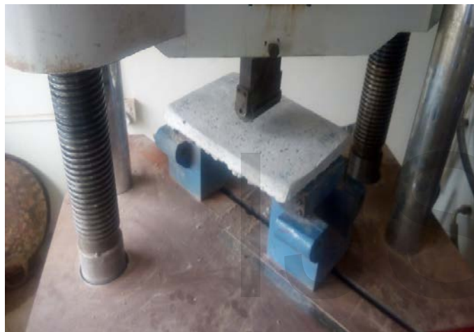
Plate 1 Specimen undergoing Flexural Strength test
